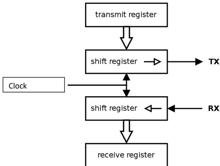
Figure 4, example UART architecture. (Source: [https://en.wikipedia.org/wiki/File:UART\\_block\\_diagram.svg](https://en.wikipedia.org/wiki/File:UART_block_diagram.svg))
